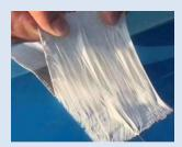
Waterproofing butyl sealant is a kind of permanent adhesive and elastic sealant which is made from butyl rubber as the theme material with tackifying resin and functional elastic body after special mixing process. It is mainly used for the coating of waterproof butyl tape, single-sided and double-sided self-adhesive waterproof roll and overlapping tape, etc.
